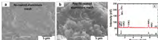
Figure 4.12 SEM images of (a) Ni-modified aluminium (Ni-Al) mesh, (b) Ppy coated Ni modified-aluminium (Ppy-Ni-Al) mesh, (c) EDS of (i) Ni-Al mesh and (ii) Ppy-Ni-Al mesh.
