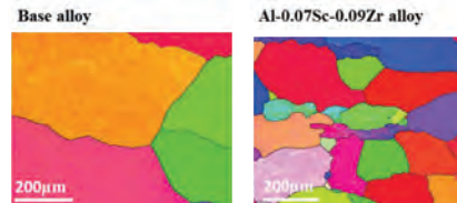
Fig.8 EBSD maps after 5% cold work and simulated brazing
