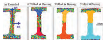
Fig.3 Microstructure of micro channel tubes after extrusion, rolling and brazing
